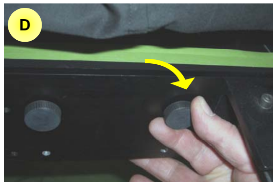
D Mount the 19RP to the backplate with the button head screws or the 1/4-20 thumbscrews.
