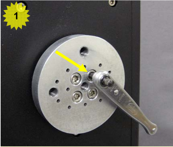
Fasten Spacer Hub to Tilt Shaft with socket head bolts
