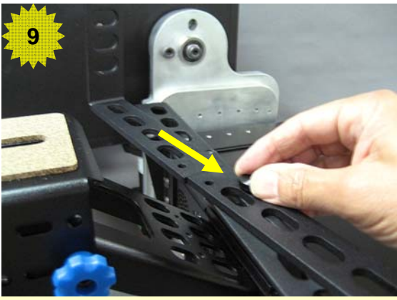
9 Attach lens frame to prompter display with 4 thumbscrews
