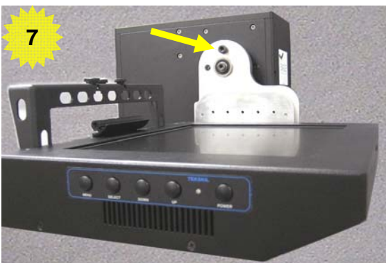
Remove Lock Bolt, rotate DBC back to horizontal and insert Lock Bolt into Spacer Hub at 12 o'clock
