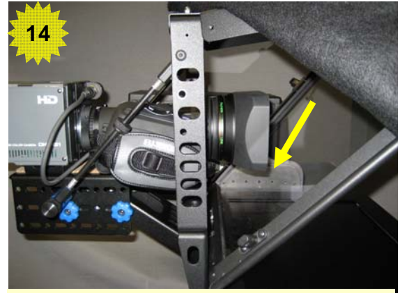
14 Attach camera to camera mount and position forward until lens is 1/2 inch from beamsplitter
