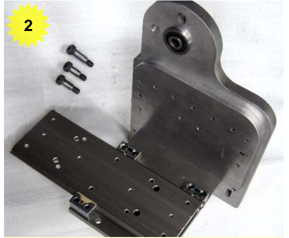
Pre-assembled Dynamic Balance Cradle (DBC) Shown with Pivot Bolt (1) and Lock Bolts (2)
