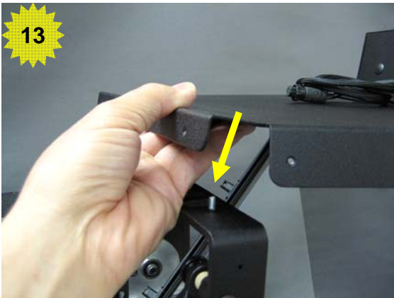
13 Attach hood panel to top edge of beamsplitter frame and secure to lens frame with 2 acorn nuts
