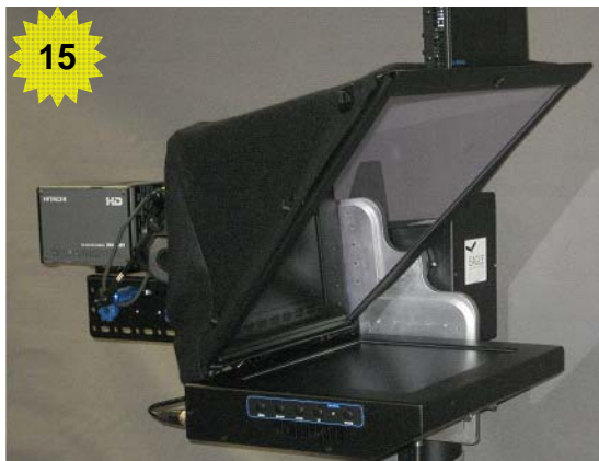
Fasten shroud and tension stabilizing arms – do not over tighten. Your Pan Tilt unit is ready to balance.
