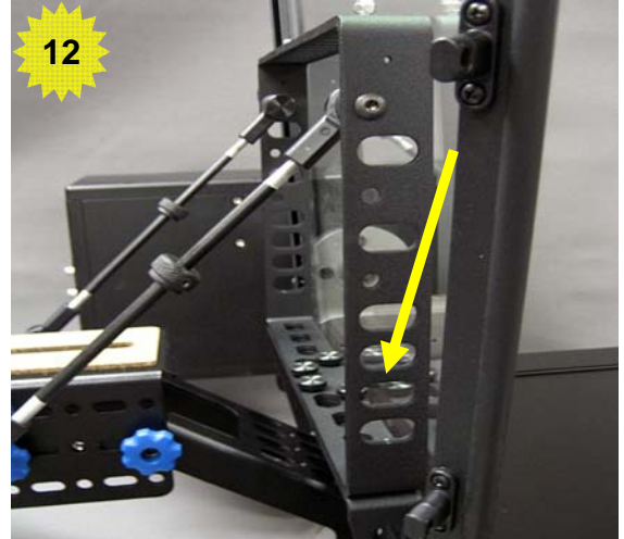
12 Insert beamsplitter frame vertically into pivot bracket and rotate forward to 45 degrees
