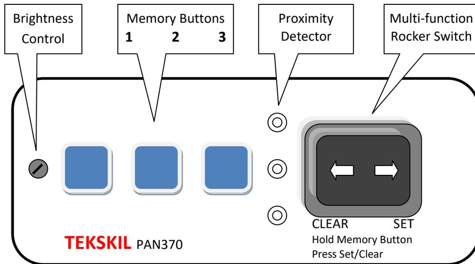
**Brightness Control** – (accessible with a small screwdriver) Adjust the brightness and set dimming operation of the Memory Button Indicators and logo panel.
