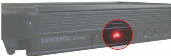
The TA90 Tally Light is a three LED array mounted to the front of Tekskil's prompter monitor. Highly visible to the Talent immediately below the prompt text, this configuration provides instantaneous 'on-air' information. This is our most economical and popular single stage tally solution.
