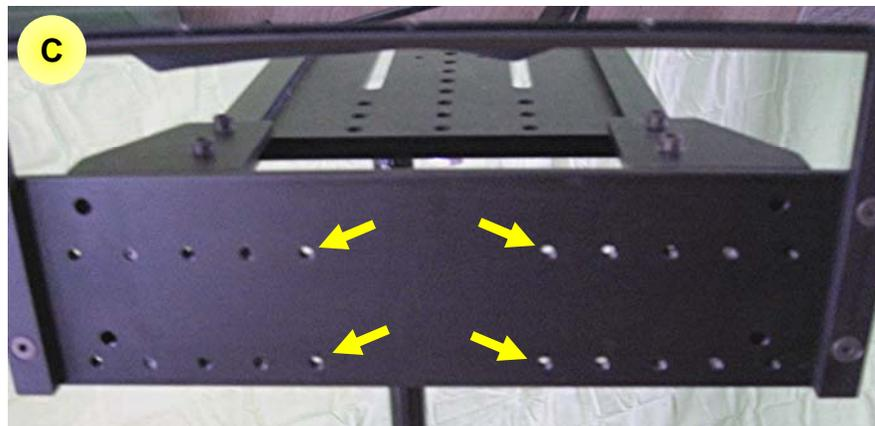
**C** Use a 1/4" drill bit to clear the threads from the four centermost holes in the backplate - these are the mounting holes for the new LCD display.
