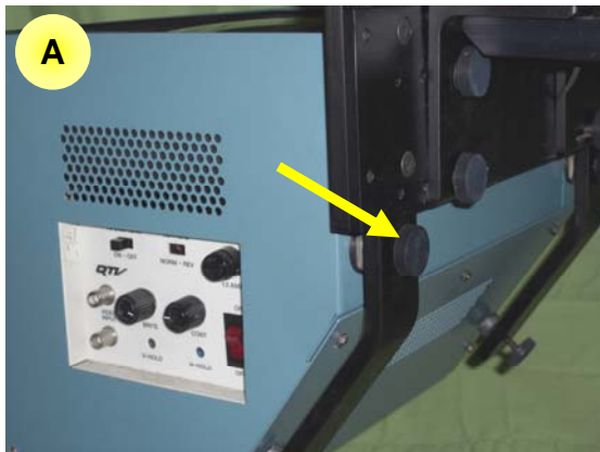
A Start by removing the old CRT. There are 2 thumbscrews to unscrew - they can be used to mount the new display.
