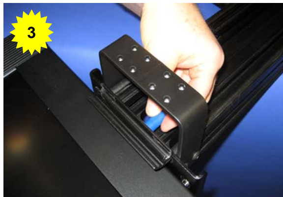
Dock Prompter Display studs (2) into the Rail plate keyholes and lock in place with the blue barrel nut
