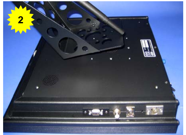
Attach the Aux Display Bracket to the underside of the Prompter Display with the 4 thumbnuts
