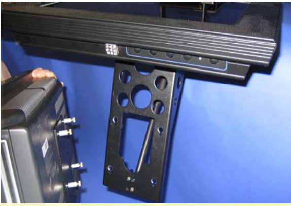
Dock the Auxiliary Display to support bracket by inserting the 4 knurled thumbnuts into the keyholes
