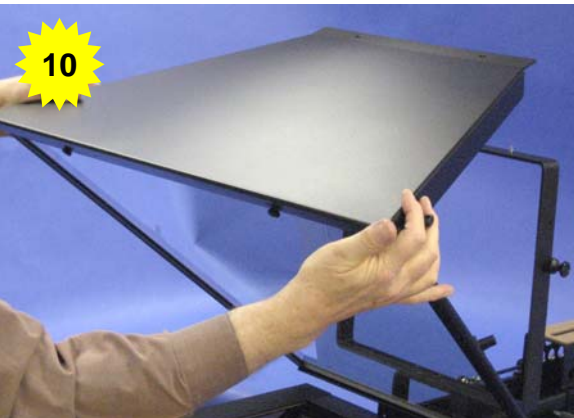
Install top panel – fasten the front thumbscrew and top knurled nuts. Support the glass during this step
