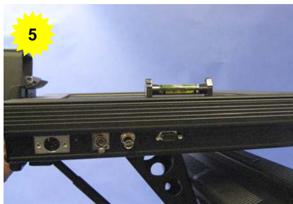
Level the Prompter Display by extending Aux Display support arm (turn counterclockwise – step 4 detail)
