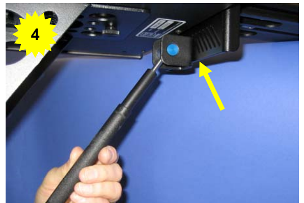
Slide upper end of Aux Display support arm into the slot in the Rail face plate and secure with thumbwheel
